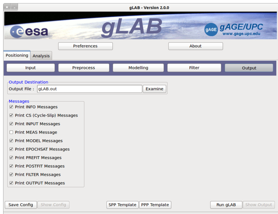
Figure 1.4: Output panel showing the different printable messages with information on the internal computations.
