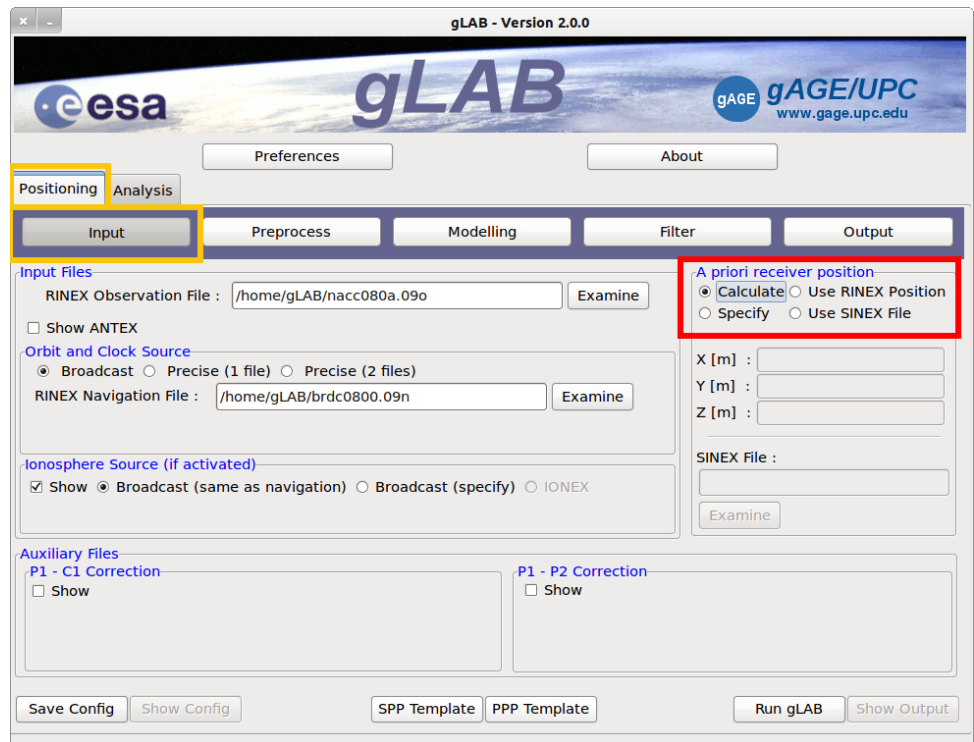
Figure 1.23: gLAB panels. Configuration to process trajectories with the option [Calculate] in the 'A priori receiver position' box set.
